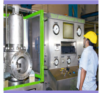
Safety Relief Valve Testing Machine
